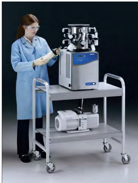
FreeZone 1 Liter Benchtop Freeze Dry Systems offer an economical solution for processing light sample loads or dedicated use by one researcher.
